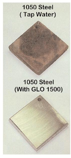
GLO 1500 removes rust and corrosion, while adding a protective coating. It is not as aggressive and fast-acting as GLO 2000 (which works in minutes), but then it only requires one application. The two samples of 1050 Steel above were "stress tested" in solution at 120 C. for 3 weeks. Despite this abuse, the amazing results are self-evident
